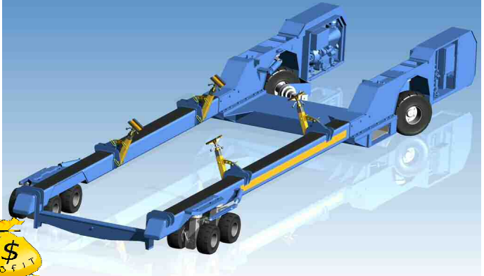
Transporter HK25 equipped with tilt adjustable telescopic supports and supporting beams
