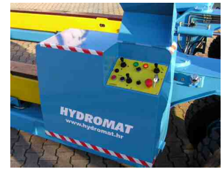
Local control panel
